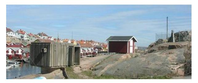
**Figure 5.** Smögen, a mareograph (hut to the left) also combined with CGPS (monument to the right) and absolute gravity platform (hut in the middle).
