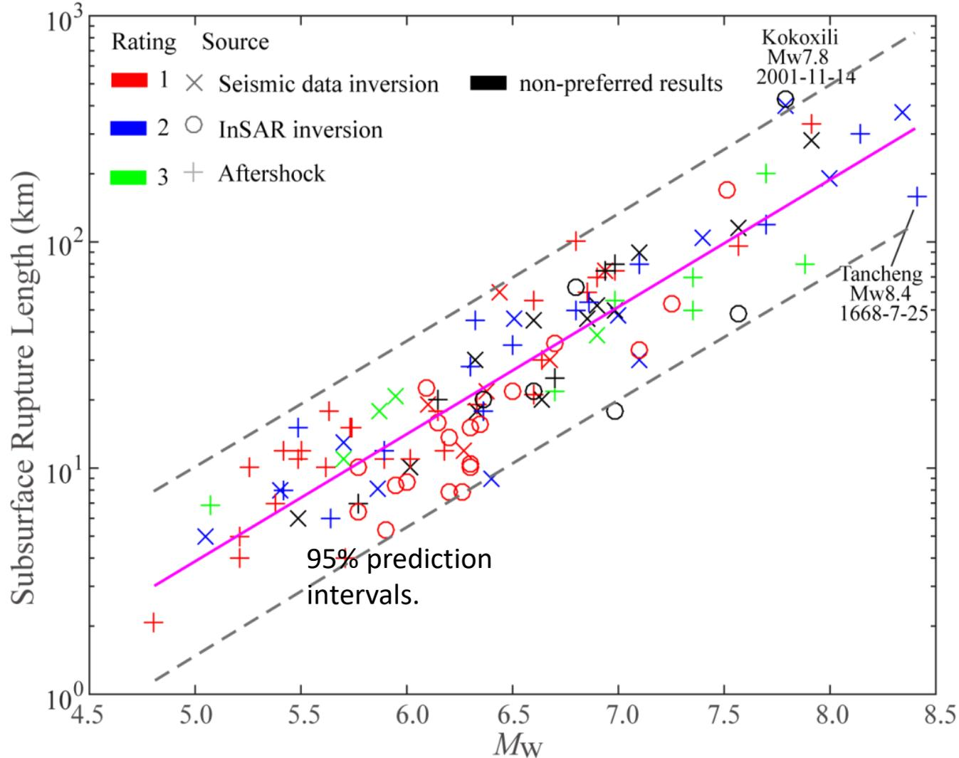
The result shows that the source model from the three methods can be used together.
