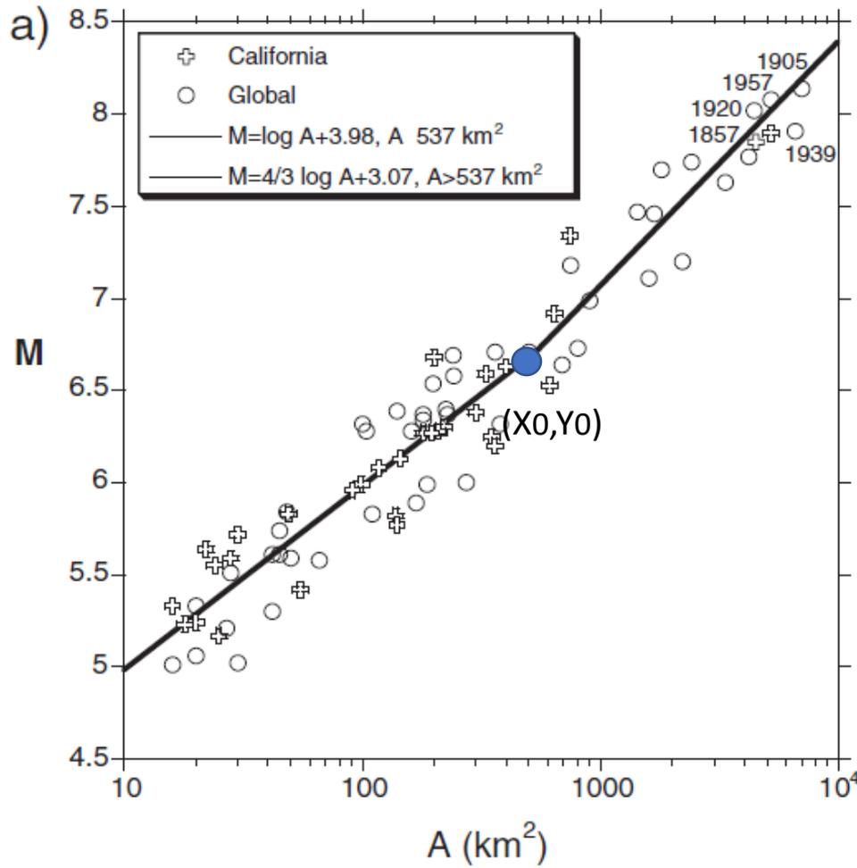
Fault rupture is width limited by the seismogenic Depth.
